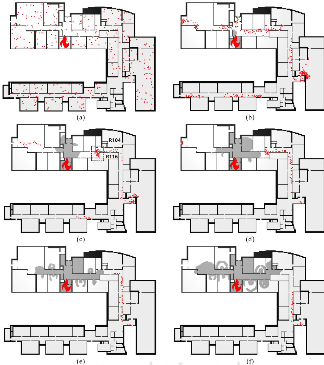
Figure 8. Agent-based evacuation simulation considering smoke spreading; (a) t=0 , (b) t=50 , (c) t=100 , (d) t=150 , (e) t=200 , (f) t=250
